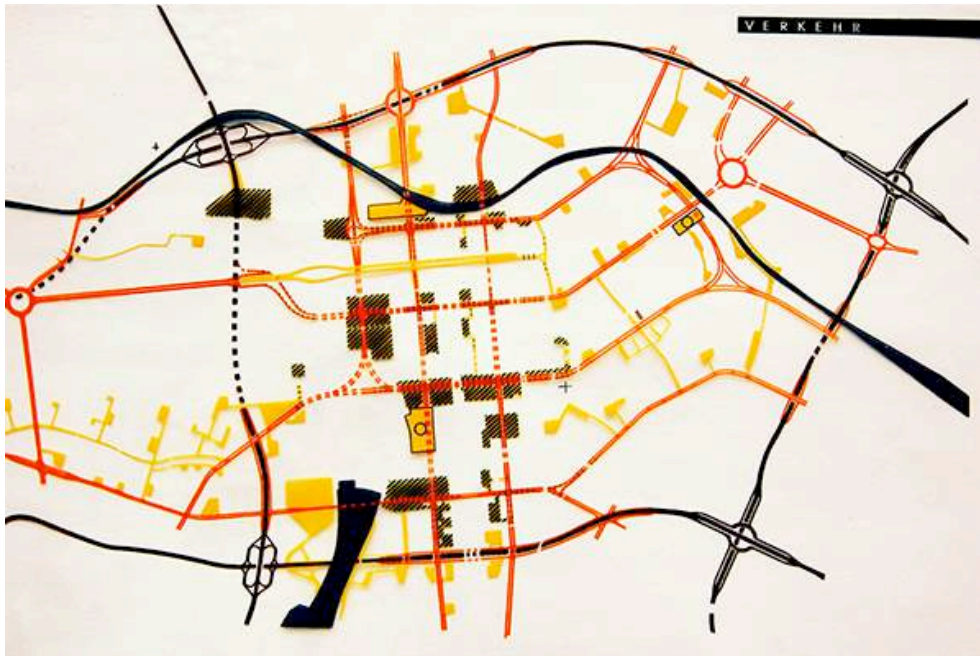
Fig. 27. One of the second prizes (Hartmann). He proposes tunnels to connect 17 Juni Strasse with Französischerstrasse as well as to underpass the new Leipzigerplatz. A traffic distributor is placed directly in front of the Reichstag.
