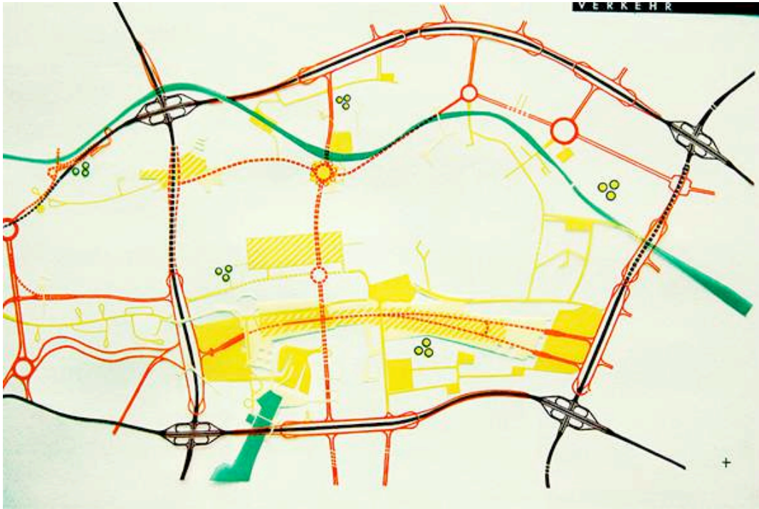
Fig. 30. One of the second prizes (Scharoun). To avoid the interference of vehicle circulation at ground level he proposes more than six miles of tunnels. One goes under Unter den Linden and the Spree to return to surface on the northeast side of the Museum Insel. A second one connects the West Tangent to the center. A third follows all along Leipzigerstrasse. There are two traffic distributors underground.
